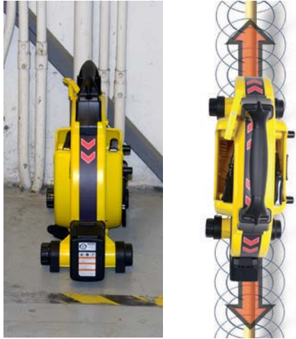
Figure 4 – Induction with RIDGID SeekTech ST-33QR
