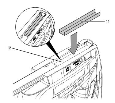
4. Alternatively, the magazine (12) can also be filled with wire nails (10) – insert them on the left-hand side. Observe the mark (13) on the left-hand side of the magazine slider that indicates the guiding groove for the wire nails. Insert the wire nails in the magazine with their heads pointing downwards.
