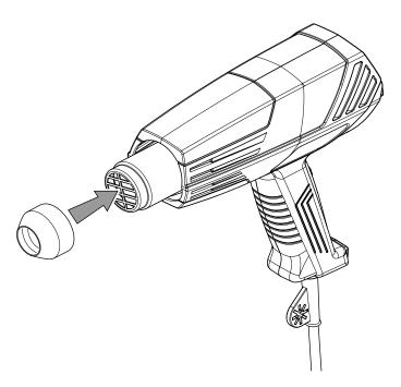
2. Make sure that the attachment nozzle is plugged on all the way and fits tightly.
